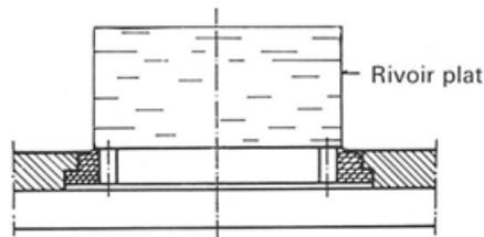
Fit the new differential crown 1476 by forcing with a flat riveting tool slightly smaller in diameter than the crown, using a turning movement.
