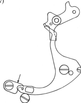
5.6.2. Set chronograph in stop position. Check that the valet for minute recorder clamp 1761 has some play between the minute recorder clamp (2 pieces) 1762 (Adjustment by eccentric of valet for minute recorder clamp 1761.)
