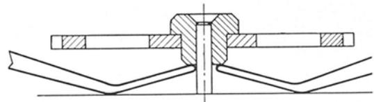
2.3.4. Unscrew the screw of pusher-stem for zero action 2482.
