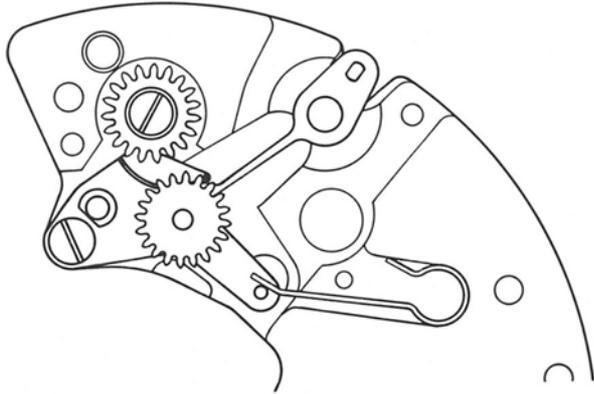
Grease (2.01) function of spring for date corrector lever 1576 on date corrector lever 1568.
